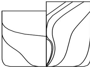
Fig. 1 Body plan of the post-Panamax container ship
