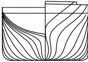
Fig. 9 Body plan of the ITTC ShipA-1 containership
