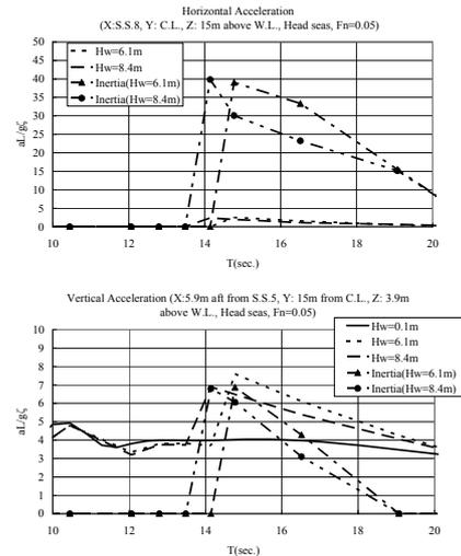
Fig. 24 Effect of wave height on the response amplitude operators of horizontal (above) and vertical (below) accelerations (Ogawa et al., 2007B)
