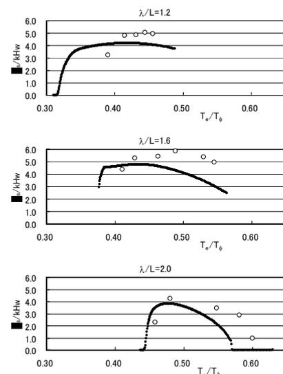
Fig. 17 Influence of encounter period on the amplitude of parametric rolling in regular head waves with  $H=0.11\text{m}$  (Taguchi et al., 2006C)
