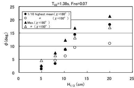
Fig. 4 Influence of significant wave height on parametric rolling in long-crested irregular head waves with  $T_{02}=1.38$ sec. (Taguchi et al., 2006B)
