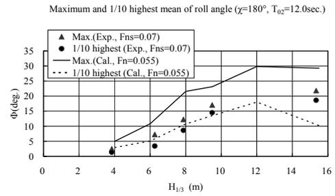
Fig. 23 Comparison of maximum roll angle of parametric rolling in long-crested irregular head waves with  $T_{02}=12.0sec$ . (Ogawa, 2007)
