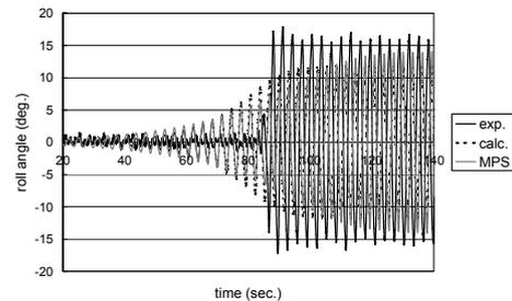
Fig. 30 Comparison of roll motion between model experiment and calculations in regular head waves  $\lambda/L=1.6$  and  $H/\lambda=0.033$  (Hashimoto et al, 2007B)
