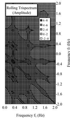
Fig. 27 Trispectrum of roll and pitch motions in regular head waves with  $f_3=0.32\text{Hz}$ ,  $H/\lambda=1/20$  and  $\lambda/L=1.6$  (Iseki, 2007)
