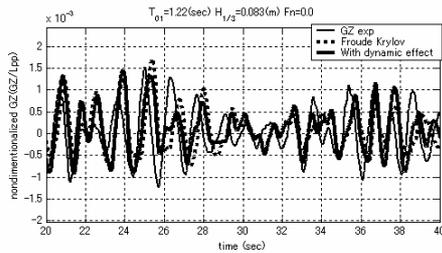
Fig. 20 Comparison of GZ variation in long-crested irregular waves with  $H_{1/3}=0.083m$  and  $T_{01}=1.22sec$ . (Hashimoto et al., 2007A)
