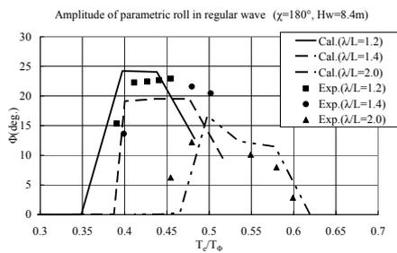
Fig. 22 Comparison of steady amplitude of parametric rolling in regular head waves with  $H=8.4m$  (Ogawa et al., 2007A)
