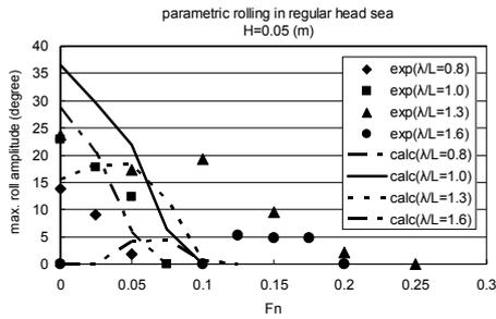
Fig. 18 Comparison of maximum roll amplitude of parametric rolling in regular head waves with  $H=0.05m$  (Hashimoto et al., 2007A)
