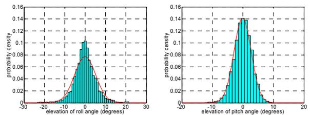
Fig. 7 Probability density functions of instantaneous roll and pitch angle in short-crested irregular waves (histogram: experiment; line: Gaussian distribution) (Hashimoto et al., 2006A)
