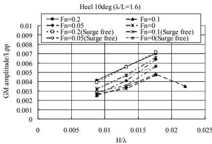
Fig. 12 Influence of surge motion on roll restoring variation in regular head waves with  $\lambda/L=1.6$  (Ogawa et al., 2007A)
