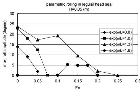
Fig. 8 Maximum roll amplitude of parametric rolling in regular head waves with  $H=0.05m$  for the PCTC (Hashimoto et al., 2007A)
