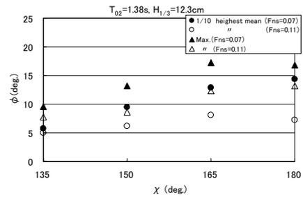
Fig. 5 Influence of encounter angle on parametric rolling in long-crested irregular waves with  $H_{1/3}=12.3$ cm and  $T_{02}=1.38$  sec. (Taguchi et al., 2006B)
