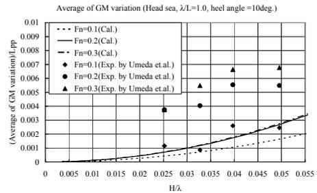
Fig. 15 Comparison of mean of GM variation in regular head waves with  $\lambda/L=1.0$  and heel angle of 10deg. (Ogawa and Ishida, 2006)
