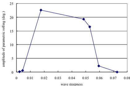
Fig. 2 Influence of wave steepness on parametric rolling in regular head waves with  $\lambda/L=1.6$  at  $\omega_e=2\omega_\phi$  (Hashimoto et al., 2006A)
