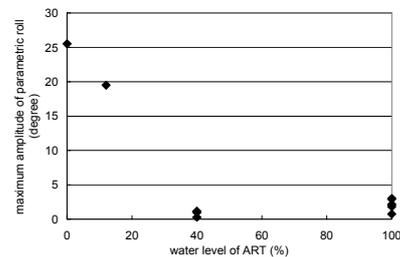
Fig. 28 Relation between water level in the ART and amplitude of parametric rolling in regular head waves at  $\lambda/L=1.3$  and  $H/\lambda=0.03$  (Umeda et al, 2008)
