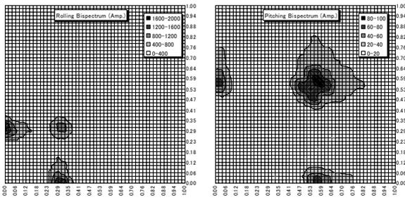
Fig. 26 Bispectra of roll and pitch motions in short-crested irregular head waves with  $H_{1/3}=0.221\text{m}$  and  $T_{01}=1.32\text{sec}$ . (Iseki, 2006)
