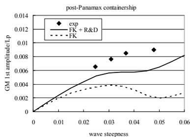
Fig. 13 Comparison of amplitude of 1st harmonic GM variation at  $F_n=0.1$  and heel angle of 10 deg. (Nakamura et al., 2007)
