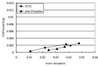
Fig. 11 Mean of GM variation at  $F_n=0.1$  and heel angle of 10deg. (Nakamura et al., 2007)
