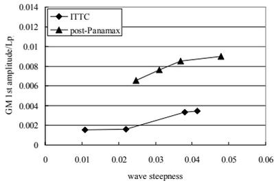
Fig. 10 Amplitude of 1st harmonic GM variation at  $F_n=0.1$  and heel angle of 10deg. (Nakamura et al., 2007)
