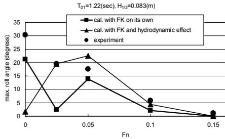
Fig. 19 Comparison of maximum roll angle of parametric rolling in long-crested irregular head waves with  $H_{1/3}=0.083m$  and  $T_{01}=1.22sec$ . (Hashimoto et al., 2007A)
