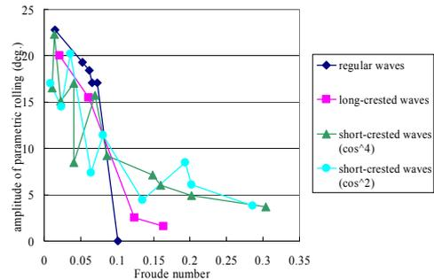
Fig. 6 Influence of ship speed on parametric rolling in regular and irregular head waves (Hashimoto et al., 2006A)
