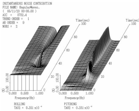
Fig. 25 Relative noise contribution to roll angle in regular head waves with  $H/\lambda=1/20$ ,  $\lambda/L=1.6$  (Iseki, 2006)
