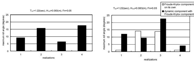
Fig. 21 Maximum roll angle of parametric rolling in long-crested irregular waves for 4 realisations (left: experiment, right: calculation) (Hashimoto et al., 2007A)
