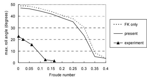
Fig. 16 Comparison of maximum roll angle of parametric rolling in long-crested irregular head waves with  $H_{1/3}=0.221\text{m}$  and  $T_{01}=1.32\text{sec}$ . (Hashimoto et al., 2006A)
