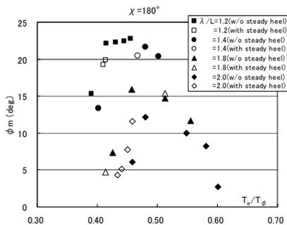
Fig. 3 Influence of initial steady heel angle on parametric rolling in regular head waves with  $H=11$ cm (Taguchi et al., 2006A)
