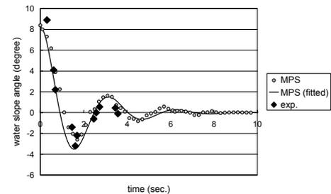
Fig. 29 Comparison of damping curve of water slope of ART between model experiment and MPS method (Hashimoto et al, 2007B)
