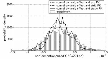
Fig. 14 PDF of restoring arm in long-crested irregular waves with  $H_{1/3}=0.057\text{m}$  and  $T_{01}=1.35\text{sec.}$  at  $F_n=0.1$  (Hashimoto et al., 2006B)
